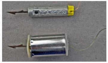
remove the barb from the skin. Detailed instructions can be found at <a href="https://help.axon.com/hc/en-us/articles/360011032994-Probe-Removal-and-Handling-Used-Probes">https://help.axon.com/hc/en-us/articles/360011032994-Probe-Removal-and-Handling-Used-Probes</a>: the cartridge safety clip is yellow and can be used to safely remove the device in the fashion identified in the images below.
